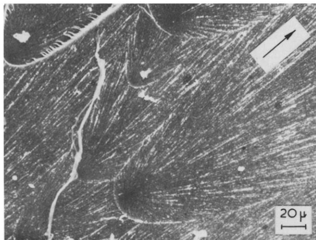
Figure 5 Parabolic marks around the smooth region. Arrow indicates crack propagation direction
